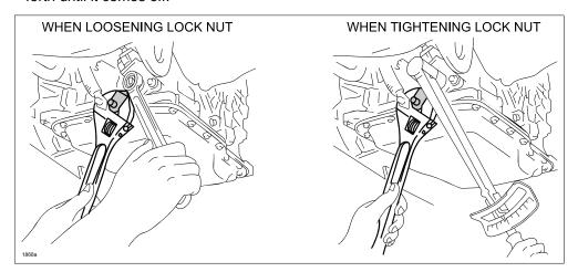
Tightening Torque: 31.4 Nm (3.2 - 4.7 kgf-m, 23.2 - 33.9 ft. lbf.)
