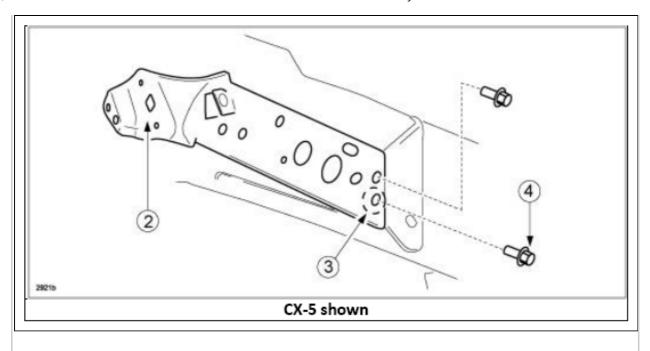
**NOTE:** Do not paint ground point (3) where attachment bolt (4) is seated.
