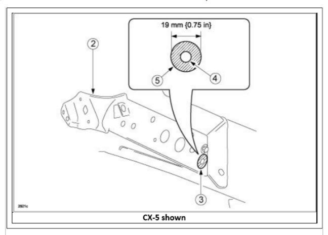
**NOTE:** After installing the bolt (4), apply touch-up paint to the exposed base material area of the front fender stay.
