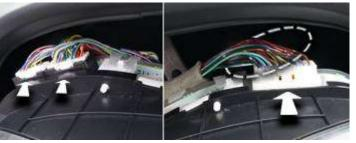
So press the small tabs with your screwdriver and at the same time grab the whole wiring bunch to pull the plug out! This maybe your only chance to get the plugs out without hurting yourself or the wiring ! Do this slowly.
