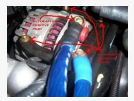
9) That's it! You're done. Reconnect the vehicle's negative battery terminal and check out the difference! Below is a shot of the "Big 3" upgraded in my car. The other wire you see coming out of the battery's positive terminal is obviously my amp's power wire.
